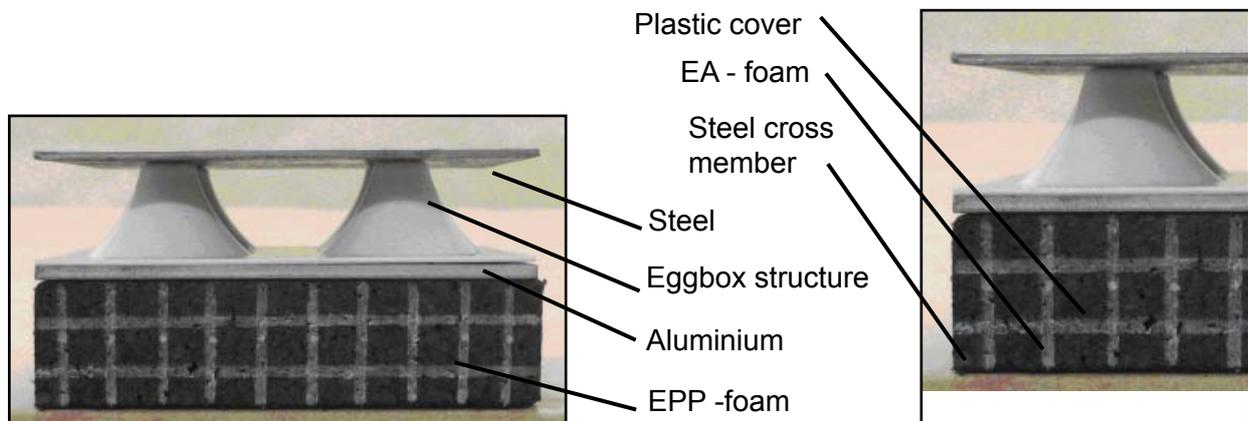
Figure 1. Architecture of an impact chain (left), Example of a vehicle front [ERN00] (right)
