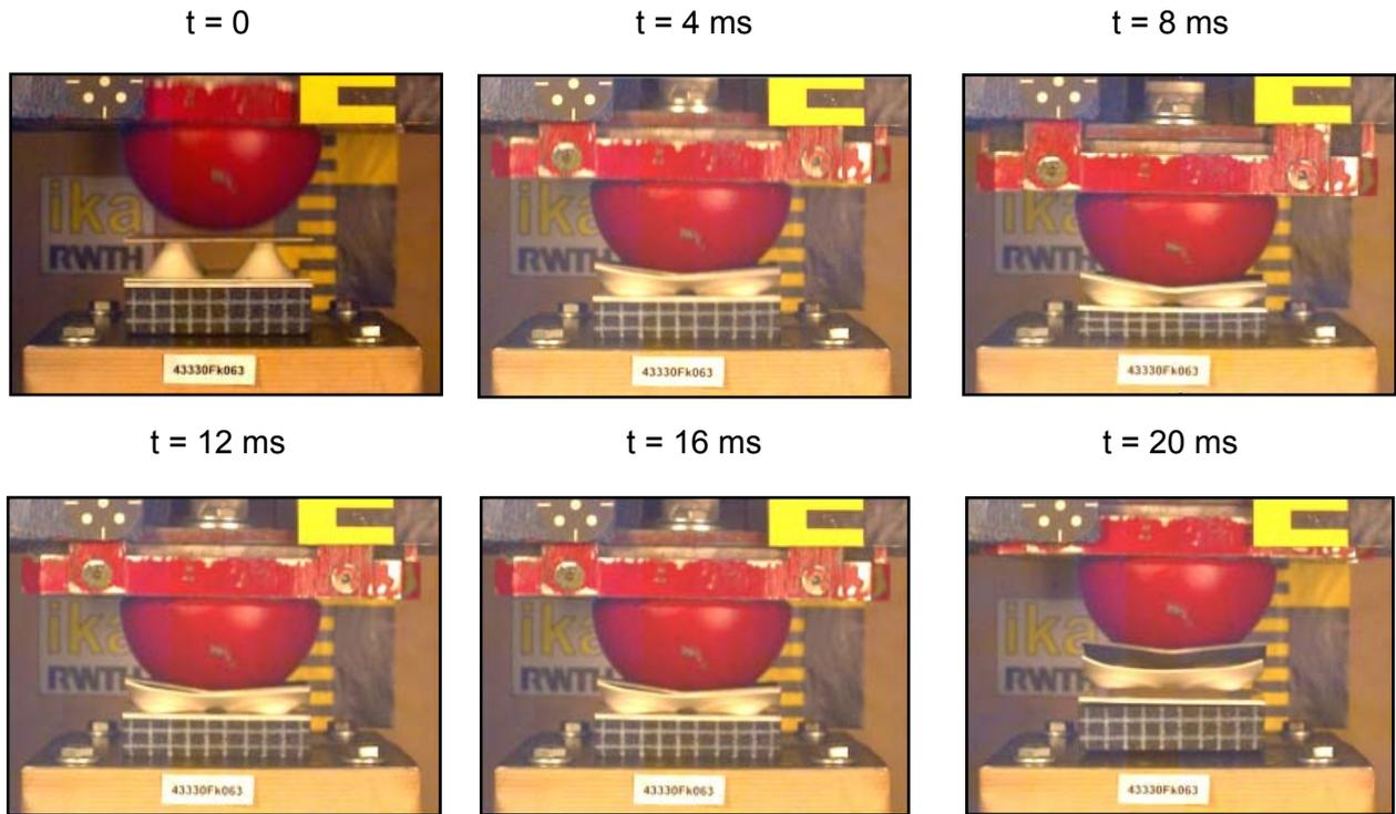
Figure 6. Test interaction chain EPP-foam aluminium eggbox structure steel
