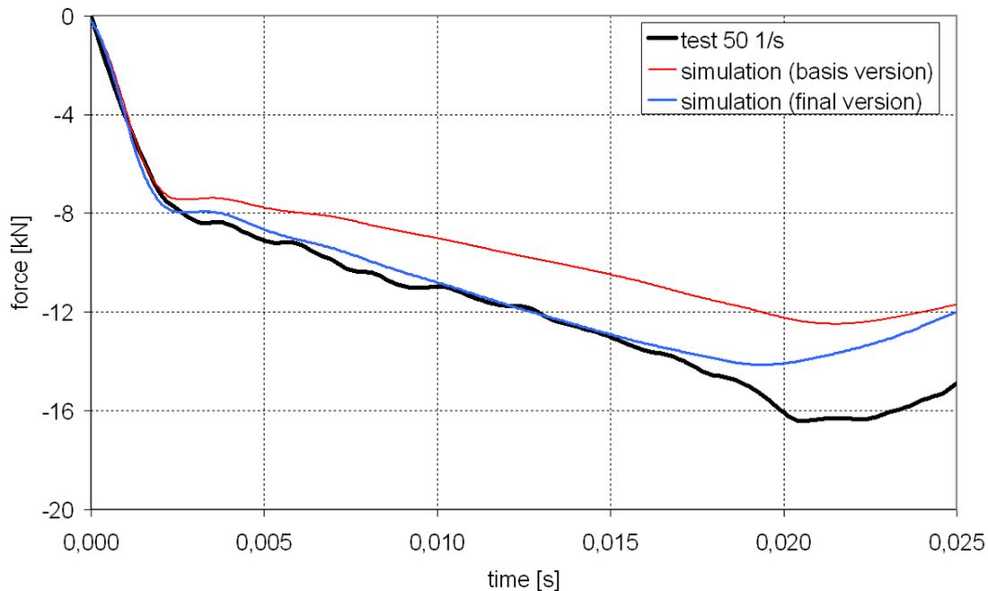
Figure 2. Delay EPP-foam strain rate 50 1/s
