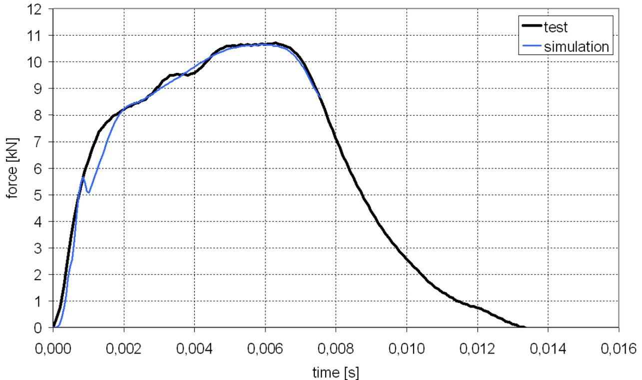
Figure 5. Comparison of simulation and test for the interaction chain EPP-steel with a hemi-spherical impactor
