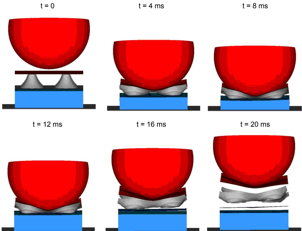
Figure 7. Simulation interaction chain EPP-foam aluminium eggbox structure steel
